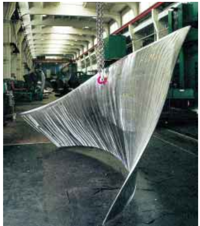
The Horse Mesa blade, machined and measured. Note the heavy skew of the blade.
