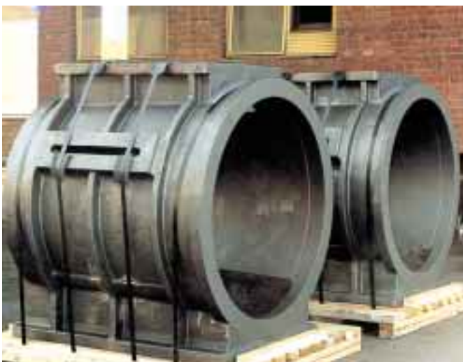
Low pressure feeder housings for pulp machine.
